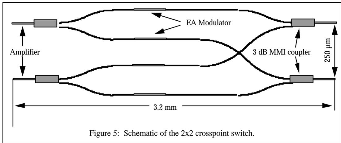
Figure 5: Schematic of the 2x2 crosspoint switch.
