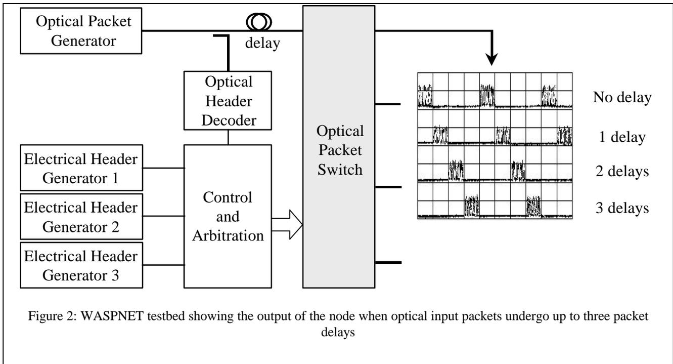
Figure 2: WASPNET testbed showing the output of the node when optical input packets undergo up to three packet delays
