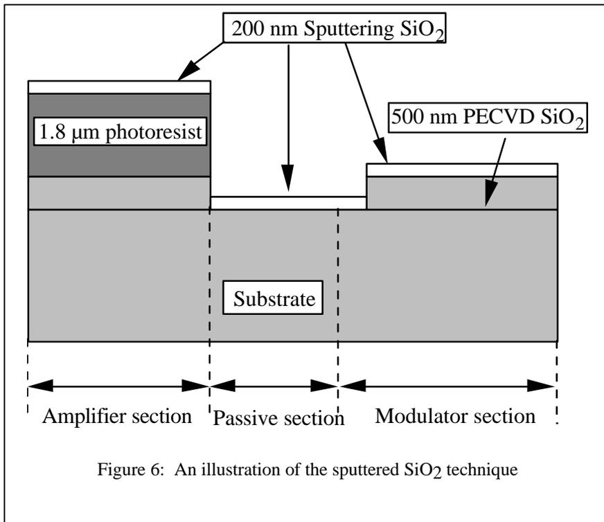
Figure 6: An illustration of the sputtered SiO<sub>2</sub> technique
