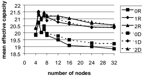
Fig. 1. Mean effective capacity for an 8-wavelength WDM ring with churn of 0.1
