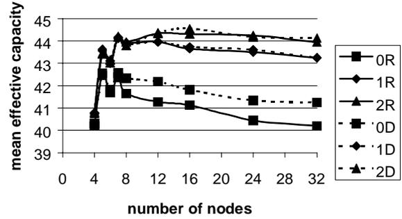
Fig. 2. Mean effective capacity for two 8-wavelength stacked WDM rings with a churn of 0.1.
