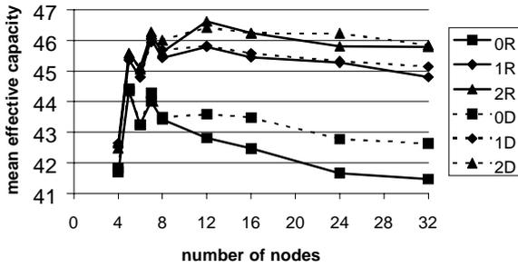
Fig. 3. Mean effective capacity for a 16-wavelength WDM ring with churn of 0.1.
