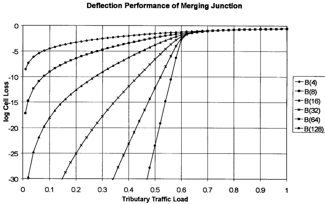
Fig. 10. Calculated deflection probability against tributary traffic load for the merging junction.
