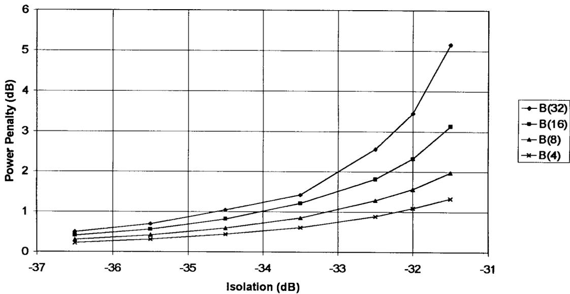
Fig. 5. Power penalty performance of the basic 2 × 2 buffered switch module for BER = 10<sup>-9</sup> and full loading plotted versus isolation performance of the switch devices.
