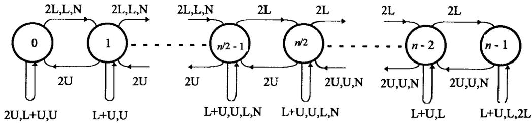
Fig. 18. State diagram for the switching module amended to allow for the possibility of fewer than two cell arrivals in a timeslot.
