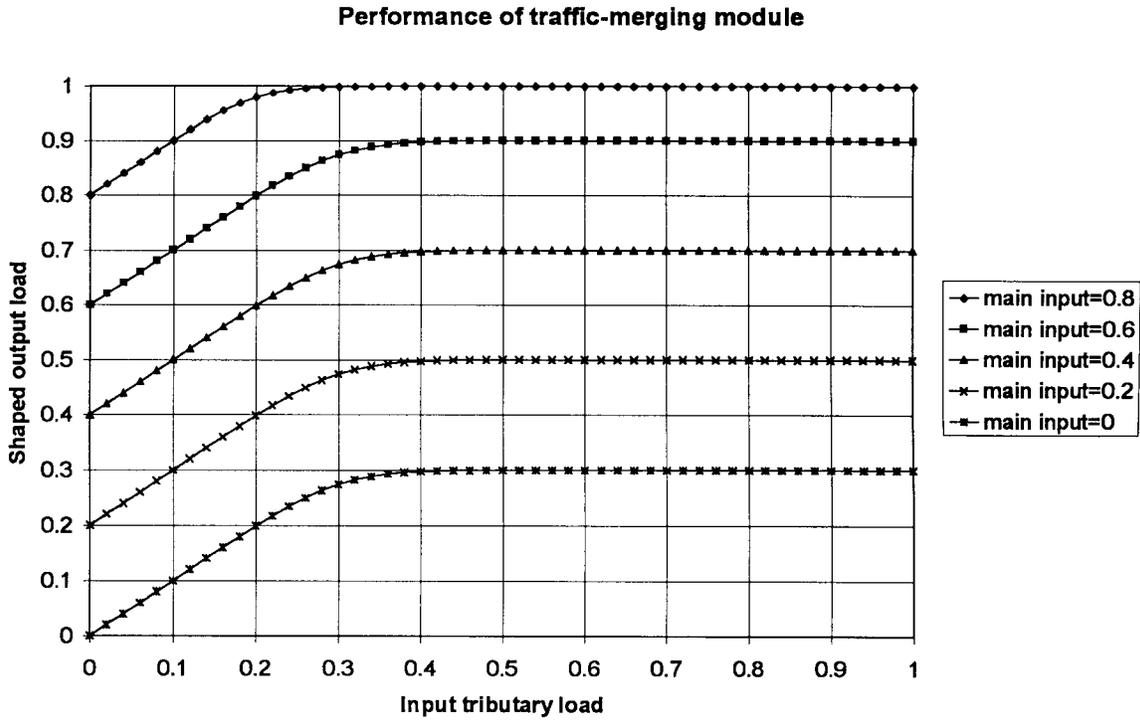
Fig. 16. Performance of a traffic-merging module ( $n = 8$ ) configured as a traffic shaping device with  $p_T = 0.3$  showing the shaped output versus input tributary traffic load, for various values of main input traffic  $p_M$ .
