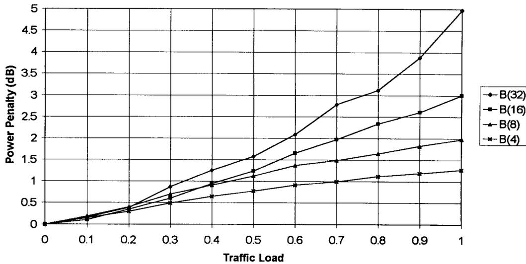
Fig. 6. Power penalties for the basic switching module for  $BER = 10^{-9}$  versus traffic load, assuming switch components with  $-31.5$  dB isolation.
