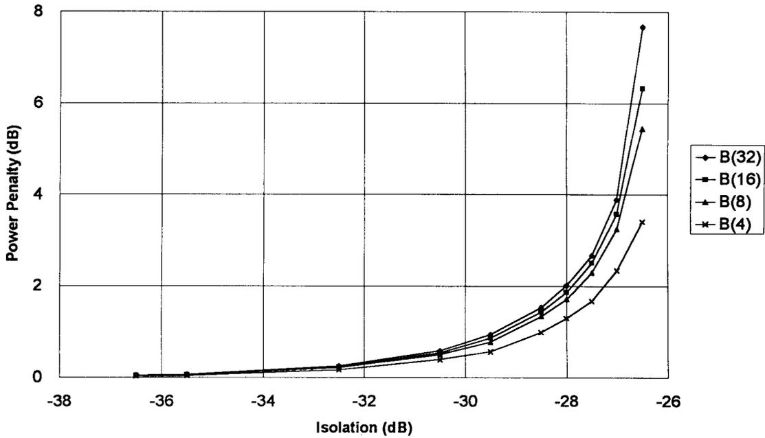
Fig. 13. Power penalties for the  $2 \times 2$  switch architecture of Fig. 12 versus isolation of the switch devices, assuming input traffic loads  $p_M = p_T = 0.5$  and  $\text{BER} = 10^{-9}$ .
