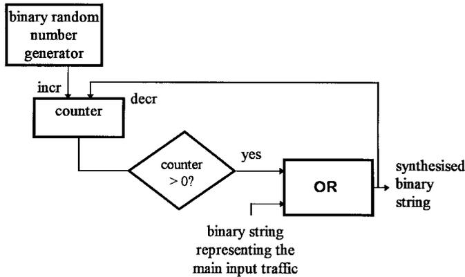
Fig. 14. Logic diagram of the algorithm to create the synthesised binary string used in the operation of the traffic shaping device. In the input and output strings, a value 1 denotes that a timeslot is filled by a cell and 0 denotes that the timeslot is empty. The binary random number generator produces one number per time slot with mean value  $p_S = 1 - p_{T \max}$ . The integer counter can cover over positive and negative values.
