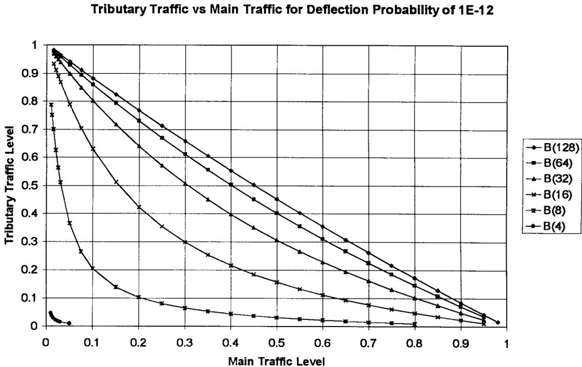
Fig. 11. Calculated maximum tributary traffic load against main traffic load for deflection probability  $<10^{-12}$ .
