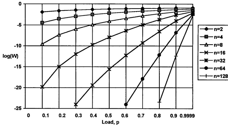
Fig. 4. Log of cell deflection probability  $\log W$  against load  $p$  for various sizes of buffering modules.
