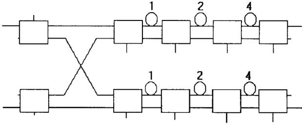
Fig. 12. A buffered switch fabric of depth eight, made up of two splitters and two combiner modules. This architecture guarantees that there are no cell deflections, but incurs a finite cell loss probability.
