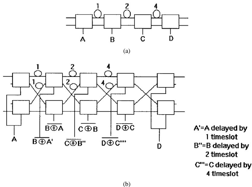
Fig. 8. The  $B(8)$  fabric with control scheme (a) undilated (b) fully dilated. The symbol “ $\oplus$ ” represents the exclusive-OR logic function.
