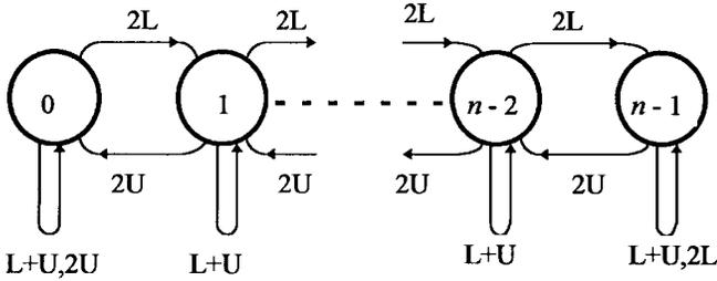
Fig. 17. State diagram of a buffered  $2 \times 2$  switch module assuming the arrival of two cells per timeslot.
