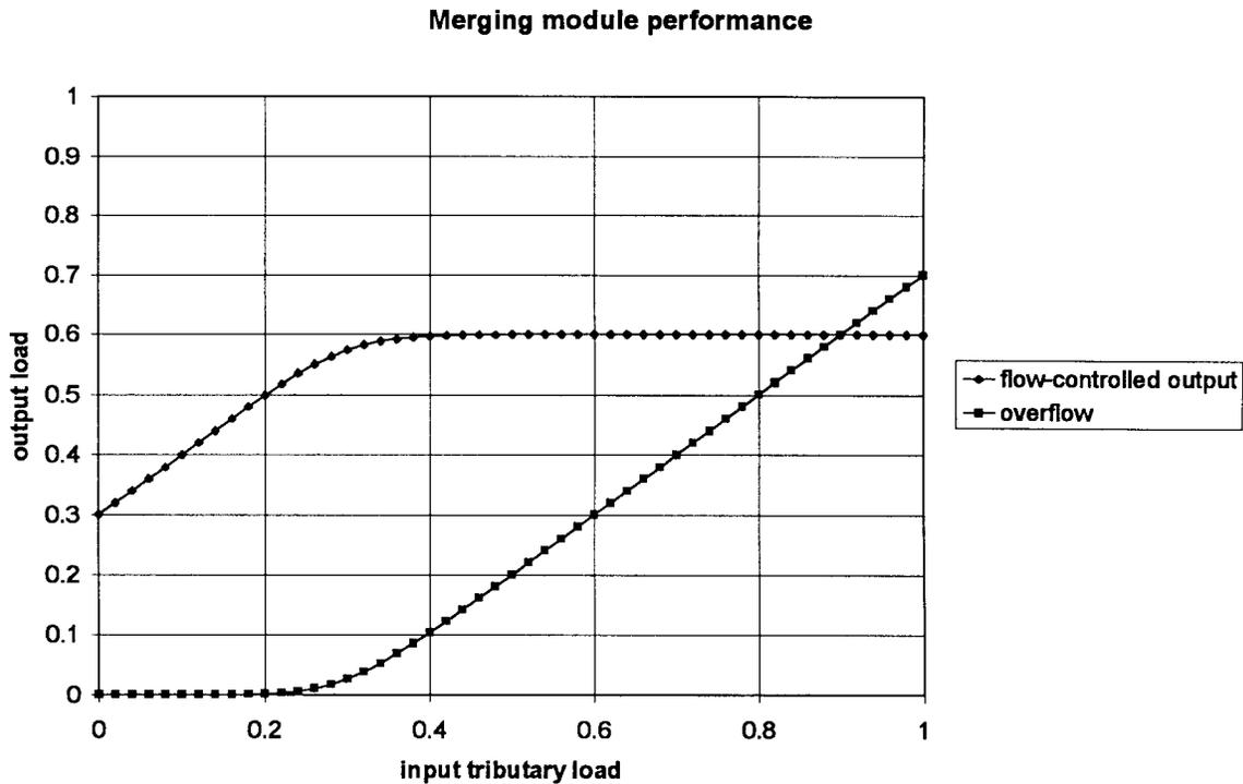
Fig. 15. Performance of a traffic-merging module ( $n = 8$ ) configured as a traffic shaping device, showing the shaped output and overflow versus input tributary traffic load. Excess tributary traffic (exceeding a preset maximum  $p_T = 0.3$ ) is diverted to the output overflow port. An arbitrary value of 0.3 is assumed for the main input traffic  $p_M$ .
