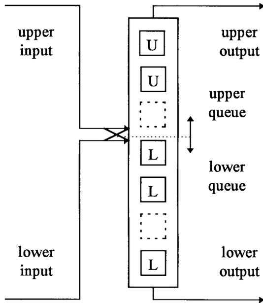
Fig. 1. Representation of the function of a  $2 \times 2$  optical contention resolution and buffering module. There are two FIFO queues; one queue is associated with the upper (U) output and the other is associated with the lower (L) output. The two FIFO queues are of variable length, but they share a common fixed length buffer and the sum of their lengths is equal to the size of the buffer. The whole module thus functions as a  $2 \times 2$  routing switch.
