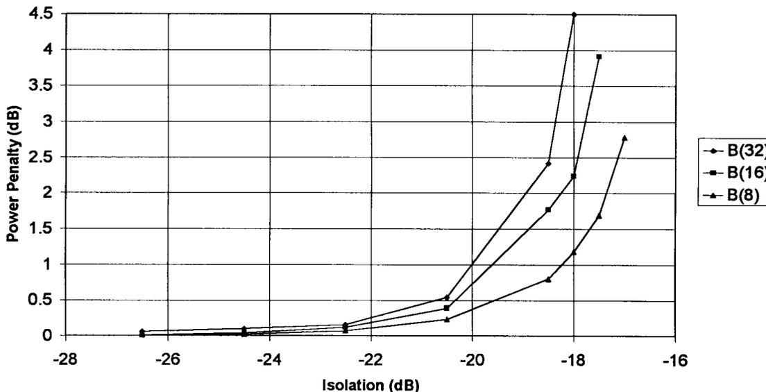
Fig. 9. Power penalties for dilated fabrics under full load assuming  $BER = 10^{-9}$  versus isolation of the switch devices.
