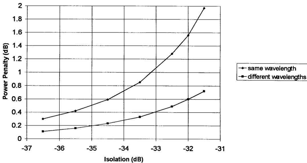
Fig. 7. Power penalties for a fully loaded  $B(8)$  plotted versus device isolation assuming  $BER = 10^{-9}$ . One curve assumes the two inputs are at different wavelengths (1550 and 1551 nm) and the other curve assumes the input wavelengths are the same.
